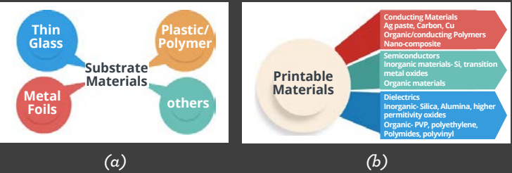
Figure 6: (a) Choice of substrate materials for printed electronics (b) Printable conductive and dielectric materials.
