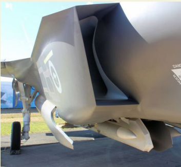
(a) Air inlet duct
