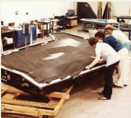
(b) Hand layup of wing section
