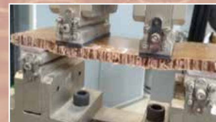
ASTM C393 (Short Beam): 4-Point-Bending
