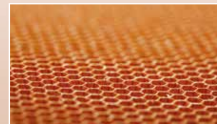
Nomex® Cores ANH4120 (Aerospace grade) and AHN7800 (Commercial grade)
