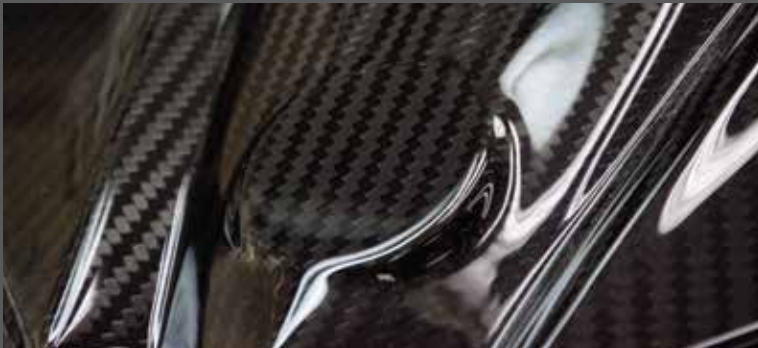
Figure 2: Composite part made with waterspot/whitespot-resistant CM14 resin system containing prepreg
