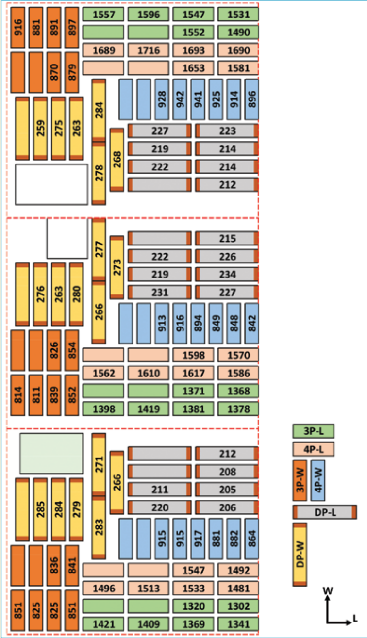
Figure 8: Maximum loads of each tests from different regions of the sandwich panel.
