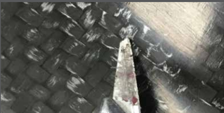
Figure 1: Carbon look composite part following incidence of white spot due to exposure to humidity
